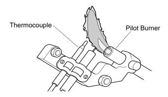
Figure 19 - Incorrect Pilot Flame Pattern
